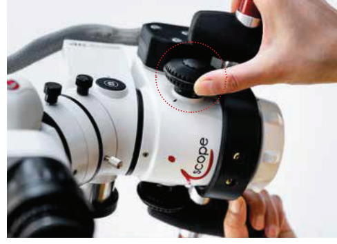
iScope Maxi 5-step magnification changer
